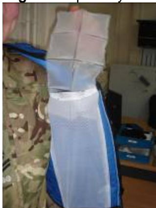
Fig 3. Cooling pack being fitted into the carrier
